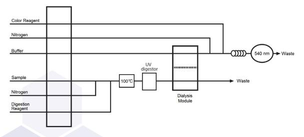
Figure 1. General Flow Diagram for Total Dissolved Nitrogen by USEPA 353.2
